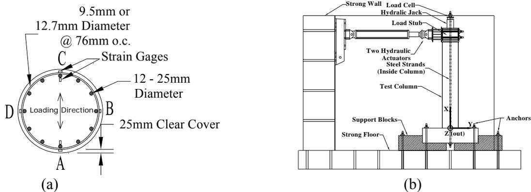
Fig. 1 (a) Column cross sectional detail and (b) test setup elevation
