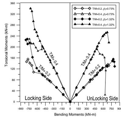
Fig. 3 Comparison of torsion-bending moments curves for various combined loading ratios
