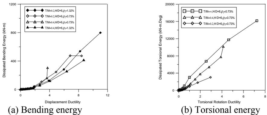
Fig. 11 Effect of spiral reinforcement ratio on energy dissipation
