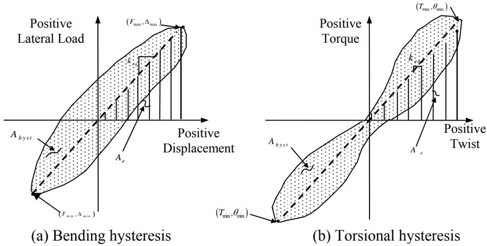
Fig. 9 Energy dissipation and equivalent definition of parameters
