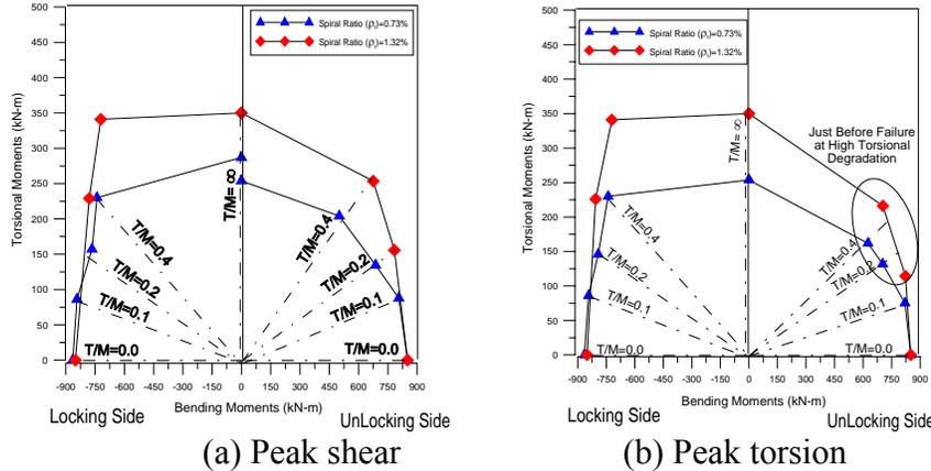
Fig. 4 Torsion-bending moments interaction diagrams
