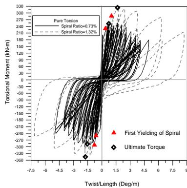
Fig. 2 Torsional hysteresis curves under pure torsion with different spiral reinforcement ratios
