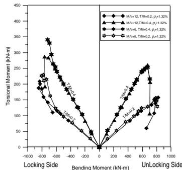
Fig. 5 Comparison of torsion-bending loading curves for two different aspect ratios
